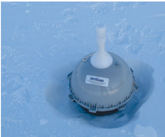
A buoy used by the International Arctic Buoy Program for ice & weather forecasts. Ocean Watch deployed three of these in the Arctic. Photo courtesy of I. Rigor, UW-APL
